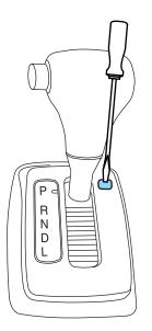
If it is necessary to use the above procedure to move the gearshift lever, it is possible that a fuse has blown or the vehicle's brakelamps are not operating properly. Refer to *Fuses and relays* in the *Roadside Emergencies* chapter.
